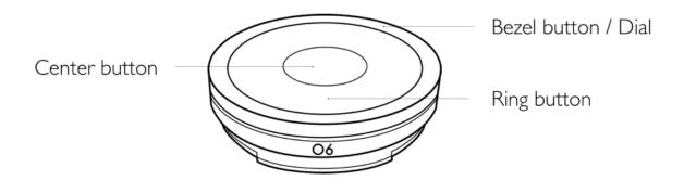
Your O6 lets you choose channels "eyes-free" through speech feedback. In addition, it has a multi-functional bezel dial and two tactile buttons:
